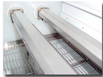
Double Air Curtain and Anti-Dragout Zone
